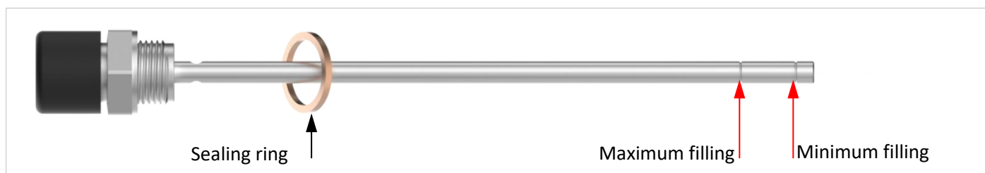
Figure 3.3.3: Breather with oil dipstick
