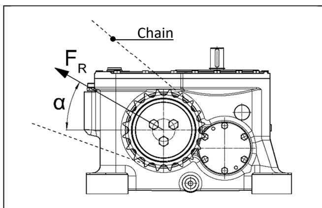
Figure 5.3.1: Radial forces and effective direction of chain
