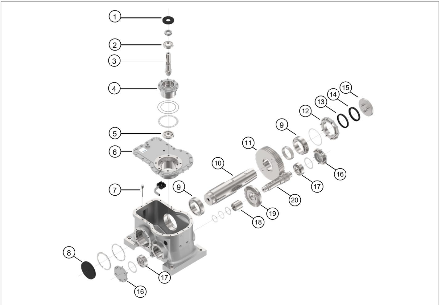
Figure 8.2: Exploded view (FTHST168.1 as example)
