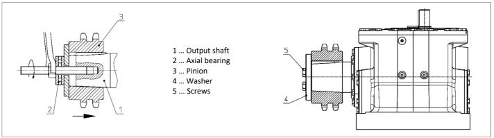
Figure 5.3: Pinion assembly for sizes FTHST168.1 and FTHST 182.1 by means of pressing/fitting
